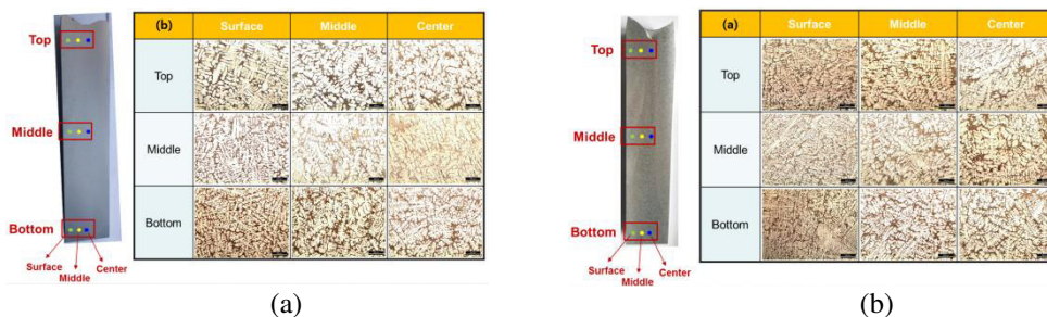
Fig. 2. Microstructures of A 356 alloy samples solidified by a) 1 casting cycle and b) 10 casting cycles.
